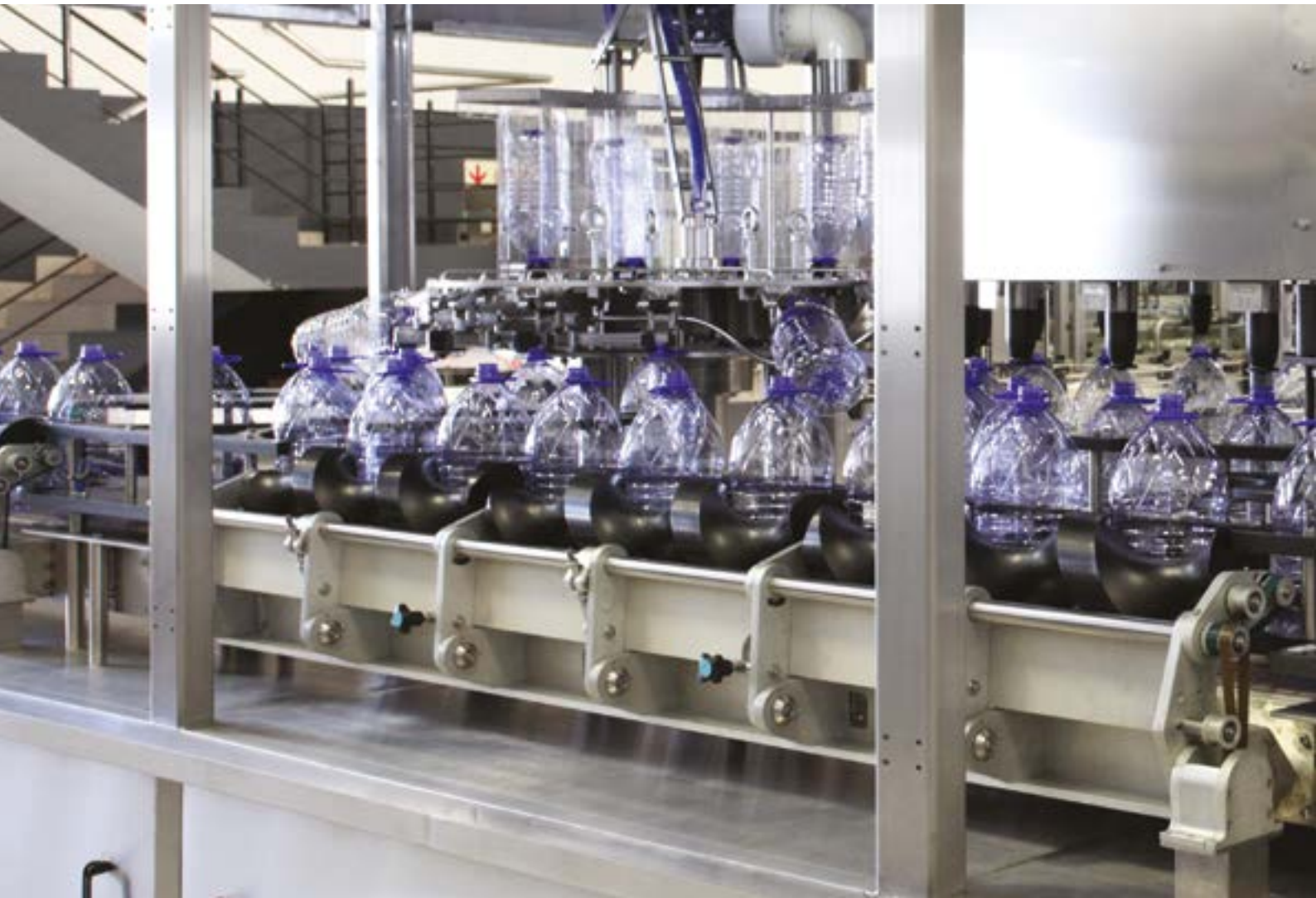
Rotary Rinser Net Weight Filler Capper Specialised for 5L bottles at 4000 bph
